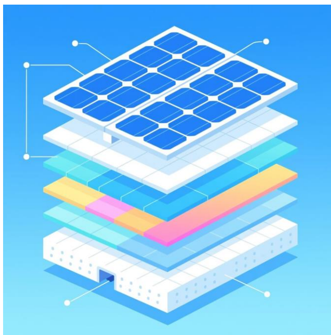
Figure 4: Structure of a photovoltaic module. Reproduced with permission ...
